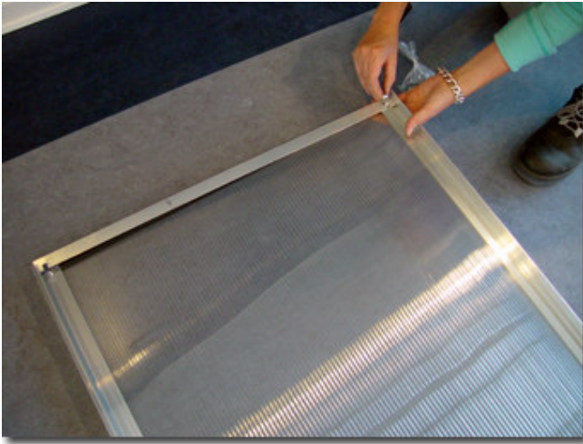
Attach the base sill 10/20 to the bottom of the wall post no. 11/21 and corner post no. 14.
